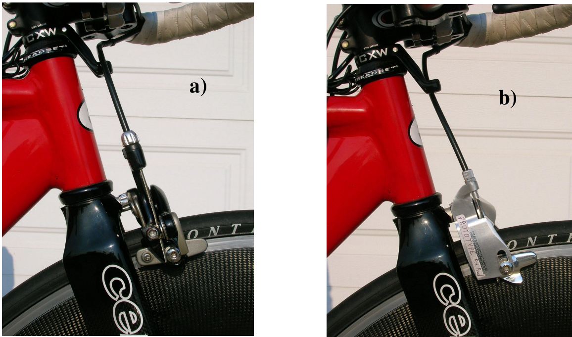
Figure 2 Side view of a) Cervelo Mach 2 brake, b) Simkins Designs Egg Brake.
